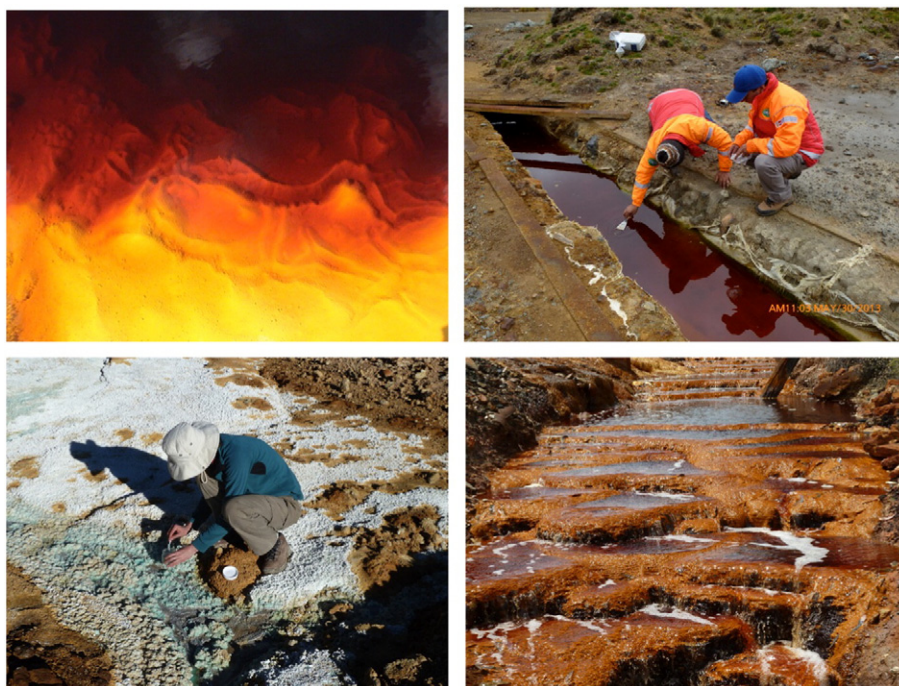
Fig. 2. Some examples of acid mine drainage. Above left: AMD pond with schwertmannite/goethite precipitating as sediment, Quilacocha tailings impoundment, Cerro de Pasco, Peru. Above right: Collection channel for the AMD solutions from Excelsior Waste Rock Dump, Cerro de Pasco, Peru. Below left: Solid AMD in form of efflorescent salts precipitating at Pan de Azúcar tailings impoundments, Argentina. Below right: Schwertmannite terraces forming in the AMD effluent from Rio Tinto mine, Spain.
